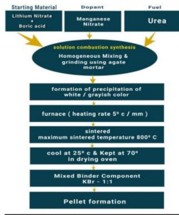
Fig. 2 - Schematic diagram of solution combustion synthesis of LTB:Mn
